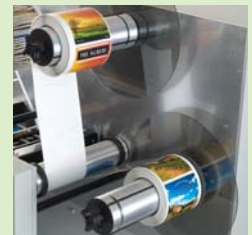
Rewinding to finished rolls
